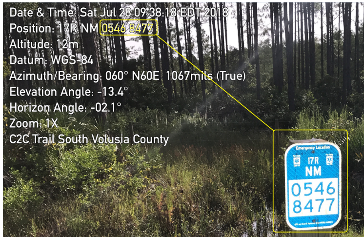
Figure 2: Emergency location marker (ELM) in Volusia County, Florida, using a smart phone app Theodolite that shows present position via USNG that matches the ELM. Photo courtesy of Al Studt.
