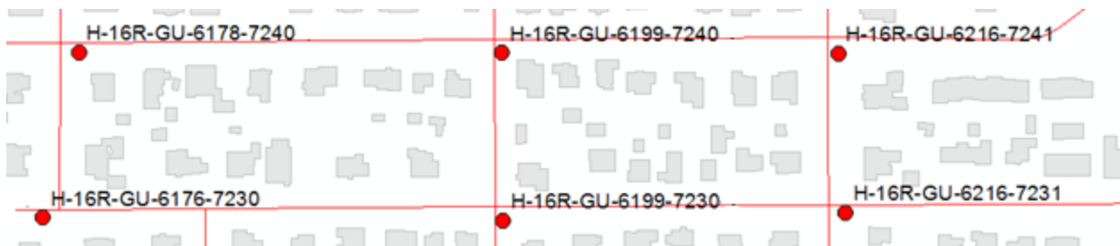
Figure 13: Hydrants showing full grid identifiers.
